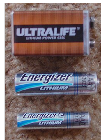
Lithium 9 volt, AA, and AAA sizes. The top object is a battery of three lithium-manganese dioxide cells; the bottom two are lithium-iron disulfide cells and are compatible with 1.5-volt alkaline cells.
